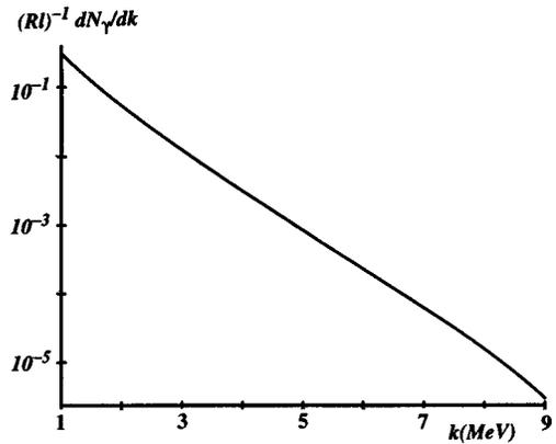
FIG. 2. The integrated-over-angle spectrum of the Bremsstrahlung radiation induced in a thin target by the MeV electrons from plasma generated by a sub-TW laser.
