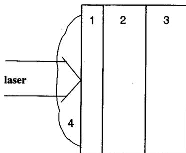
FIG. 3. Optimal target for a laser-based nuclear radiation source (not to scale). (1) a low-Z ablation layer, (2) a high-Z Bremsstrahlung converter (e.g., Ta), and (3) a neutron production layer (Be or D); (4) pre-formed plasma.
