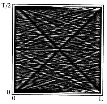
Quantum carpet woven by a particle moving with a non-relativistic velocity in a one-dimensional box. The carpet arises from the space-time representation of the probability density. As initial condition of the Schrödinger equation with the non-relativistic Hamiltonian  $H_{\rm nr}=p^2/(2M)$  we have used a Gaussian wave packet of width  $\Delta x=L/20$  and average wave number  $\bar k=10\pi/L$  located at  $\bar x=L/2$ .
