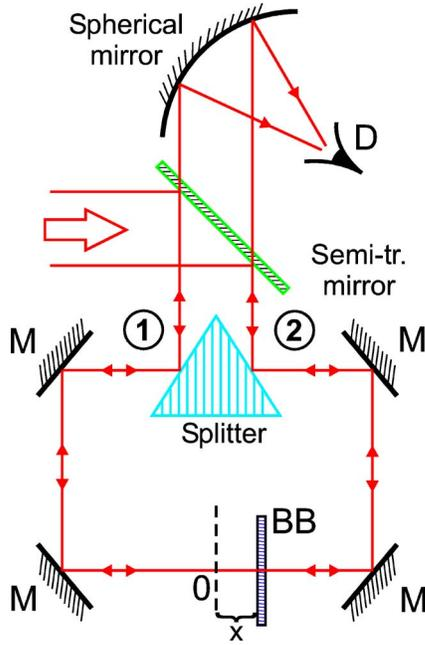
Fig. 1. (Color online) Ring (Sagnac) interferometer using a thin metallic film BB. M, metallic mirror; D, intensity detector.
