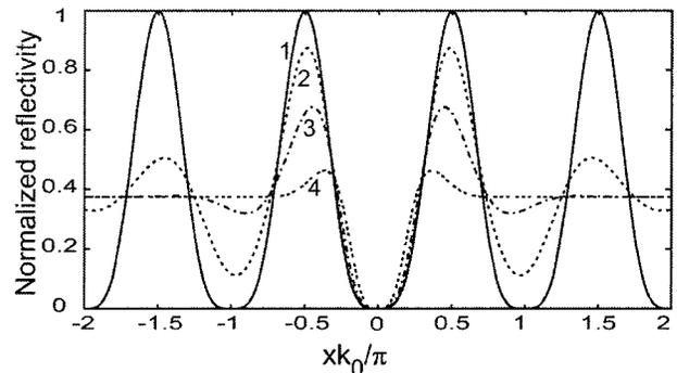
Fig. 2. Normalized refractivity of the interferometer versus normalized BB position,  $xk_0/\pi = \tau\omega_0/2\pi$ , for the broad-spectrum signal (6), for both channels. Curves: 1,  $\Delta\omega = 0$ ; 2,  $\Delta\omega = \omega_0/4$ ; 3,  $\Delta\omega = \omega_0/2$ ; 4,  $\Delta\omega = \omega_0$ .
