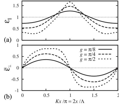
FIG. 2. Normalized electric fields at the corrugated boundary for  $\epsilon_2/\epsilon_1=6$ .
