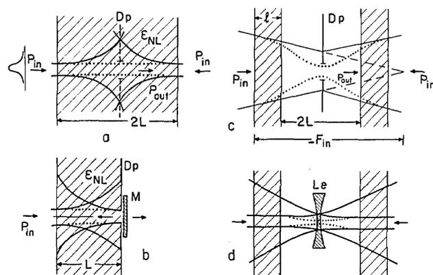
Fig. 1. Various configurations realizing optical bistability from mutual self-focusing (or self-defocusing) of counterpropagated beams. M, mirror; Dp, diaphragm; Le, lens. The solid lines show the spatial behavior of the low-power beams; the dotted lines correspond to the behavior of high-power beams after their switch into a high-transmittance state of the system.
