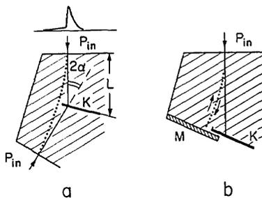
Fig. 3. Configurations realizing bistability from mutual self-bending of the light beams. M, mirror; K, knife edge.
