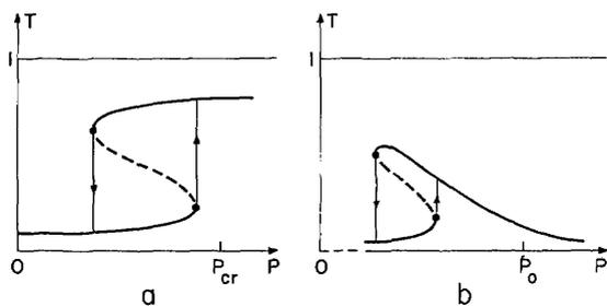
Fig. 2. Hysteresis of transmittivity  $T = P_{\text{out}}/P_{\text{in}}$  in the cases of a, self-trapping and b, external self-action.
