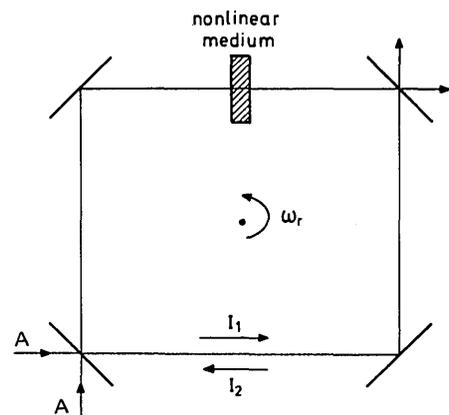
Fig. 1. Rotating ring resonator with nonlinear medium and two pumping beams of equal intensity.
