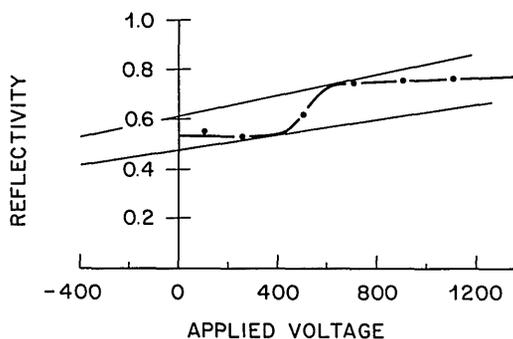
Fig. 3. Measured open-loop reflectivity as function of applied voltage. Two characteristic lines corresponding to the effect of the feedback signal have been drawn from the point on the voltage axis corresponding to the applied bias (-3100 V). The intersection of these lines with the experimental curve should correspond to the critical operating points for upswitching and downswitching.
