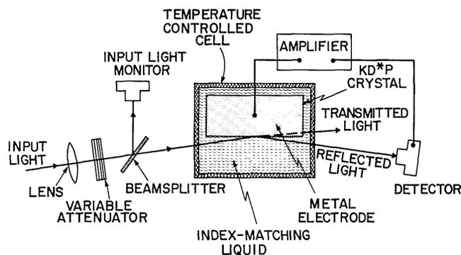
Fig. 1. Schematic of experimental setup (top view).
