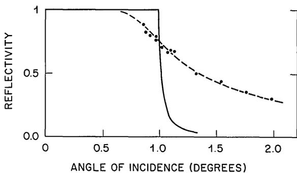
Fig. 2. Measured open-loop reflectivity as a function of angle of incidence for a temperature of 37.4°C. For comparison the computed plane-wave reflectivity (solid line) is shown for a critical angle of 1.0°.
