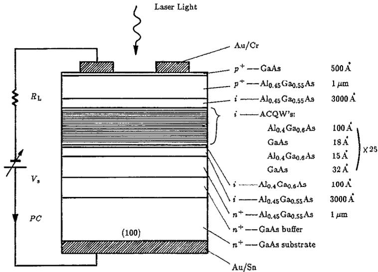
FIG. 2. The structure of a mesa *p-i-n* diode in which the intrinsic region contains ACQWs. The *i*-ACQWs layers correspond to multiple (25) QW pairs of the type shown in Fig. 1.
