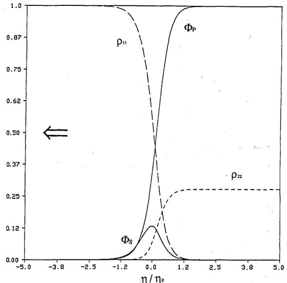
Fig. 1. Pump  $\Phi_p$  and Stokes  $\Phi_s$  photon fluxes [normalized to  $\Phi_p(\infty) = \Phi_0$ ] and the population of the ground  $\rho_{11}$  and excited  $\rho_{22}$  levels as a function of the normalized retarded time  $\eta/\eta_0$  for an IFSR soliton in He (for  $\eta_0$  see the text). The arrow indicates the direction of pulse propagation.
