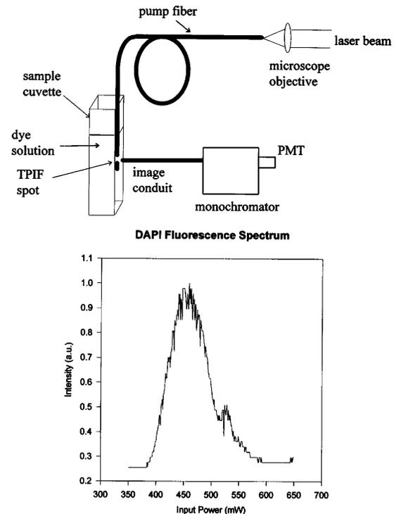
Fig. 1. Geometry used to deliver the laser light and collect the fluorescence signal. The dye-laser beam is coupled into the pump fiber and a  $10\times$  microscope objective, the fiber tip is immersed in the dye solution close to the wall of the cuvette, and then the image conduit collects the light on the other side of the cuvette wall and delivers it to the monochromator. PMT, photomultiplier tube. The detected spectrum of DAPI is also shown.
